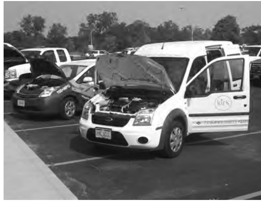
A bi-fueled Ford Transit Connect converted to run on CNG and gasoline. Photo courtesy of Kirk Energy Group, LLC.
